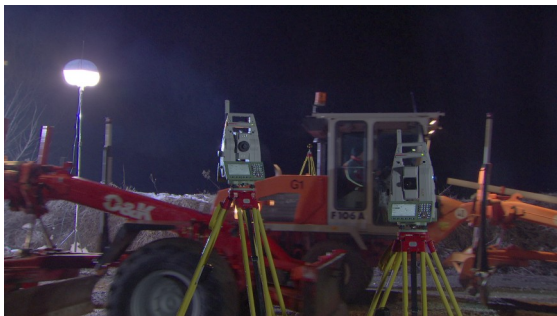
Figure 5 - Test scenario with possible negative influences on the performance of following a prism (rain, bright lights, and various targets).
